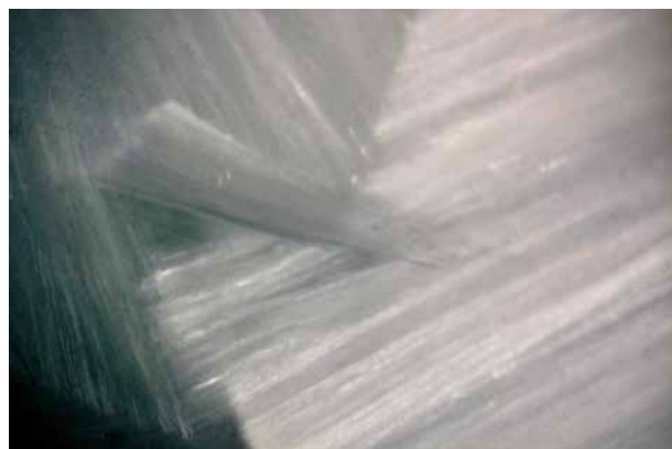
Figure 4: Fine, tightly packed, intergrown fibrous crystals arranged in a radial to subparallel pattern in opaque areas of glass-imitation of larimar. Photomicrograph by G. Choudhary; image width 5.08mm
