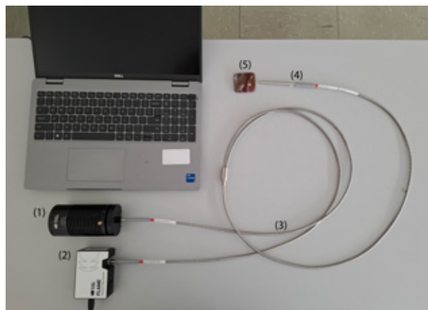
Figure 1. Fibre Optics Reflectance Spectroscopy (FORS). Ocean Optics system, described in the text.
