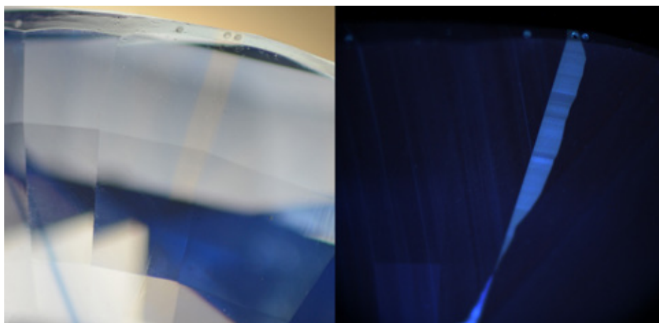
Figure 3: Thin Ta-rich (and HFSE-rich) zone in HFSE-sapphire sample 973 seen under microscope as colourless band and as chalky white zone in deep UV (DiamondView TM ).
