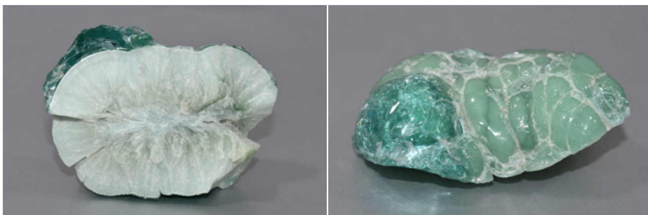
Figure 2: Rough sample of devitrified glass showing an opaque radiating pattern originating from a central core and terminating in circular edges, indicative of spherulitic growth (left). In contrast, the surface or crust of the same sample exhibits a transparent, glassy layer with a botryoidal pattern (right). Photos by G. Choudhary.
