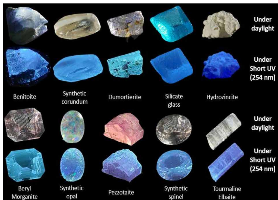
Figure 1: The ten samples investigated for BSL in daylight (top row) and shortwave ultraviolet light (bottom row). Synthetic corundum, benitoite and synthetic spinel are used as reference materials.
