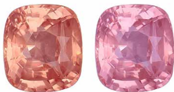
Figure 1: This fancy sapphire with unstable color is in its charged state on the left and after stability testing on the right.
