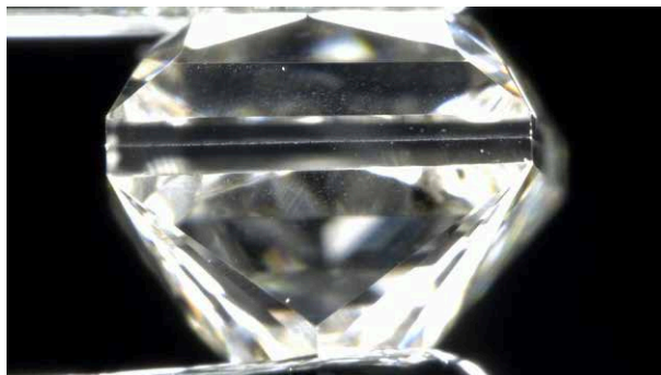
Figure 2: A boundary between natural seed crystal and the CVD growth layer was seen on the girdle.
