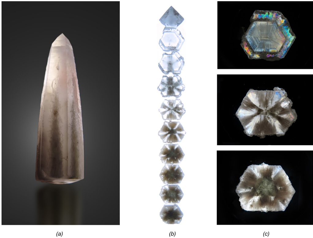
Figure 3. (a) This Tessin type quartz crystal (6x2cm) shows the distribution of inclusions under transmitted light; (b) Nine cut and polished slices of the quartz crystal (perpendicular to the c -axis), show the trapiche growth pattern and transparency changing at different parts of the crystal; (c) Three selected slices show different patterns under cross-polarised light.
