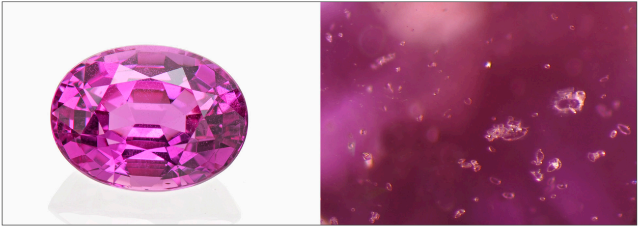
Figure 1: Pink sapphire of 7.9 ct from Ilakaka, Madagascar and photomicrograph of zircon inclusions (magnification 50x).
