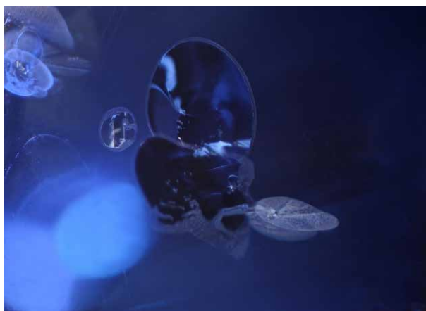
Figure 1: Discoid extension features indicating heating (at high temperatures) in this Ti-diffusion treated sapphire. Magn. 50x. Photo: M.S. Krzemnicki, SSEF
