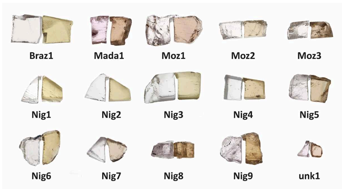
Figure 1: Mn- and Fe-bearing beryls from different localities (Braz = Brazil, Mada = Madagascar, Nig = Nigeria, Moz = Mozambique, unk = unknown) before (left) and after (right) irradiation with electrons.
