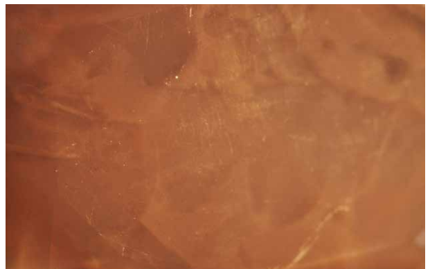
Figure 4: Grey-brown zones or areas appeared cloudy and translucent in fibre-optic lighting. Photomicrograph by G. Choudhary; image width 5.08mm
