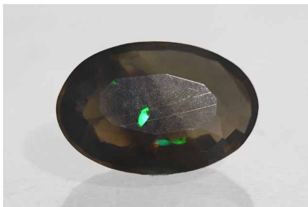
Figure 2: Weak play-of-colour effect was visible as small spots confining to grey-brown areas when illuminated with strong fibre-optic light. Photo by G. Choudhary
