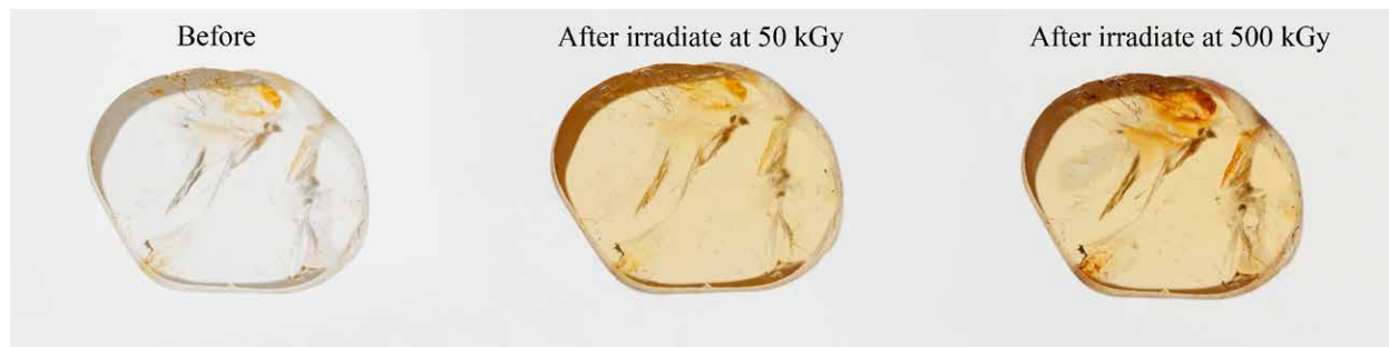
Figure 1: Color-calibrated photo of sapphire from Sri Lanka before and after gamma irradiation. Path length/thickness: 1.404 mm
