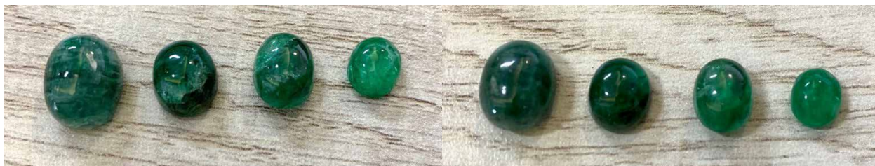
Figure 1: Pakistani emerald cabochons before (left) and after fracture filling with Johnson baby oil. Notice the fractures are not well hidden due to the difference in RI between the filler and the emerald.
