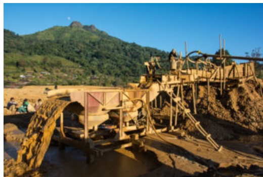
Figure 8. Stones >2.5 cm are screened off and the rest of the material passes into a jig. Photo by B. M. Laurs.
