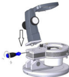
Figure 5. Sustainable LED update of a GemoLite microscope by replacing the darkfield illuminator base and keep the optical system.
