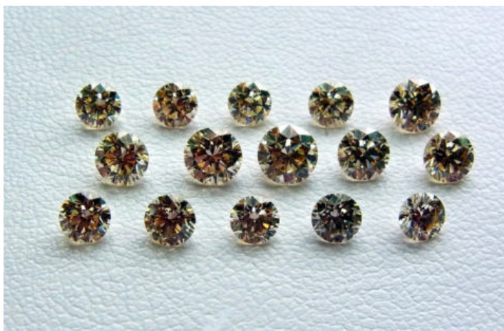
Figure 1. Fifteen type Ib yellow-brownish yellow CVD-grown synthetic diamonds(0.18-0.40ct). Photo by H. Kitawaki.
