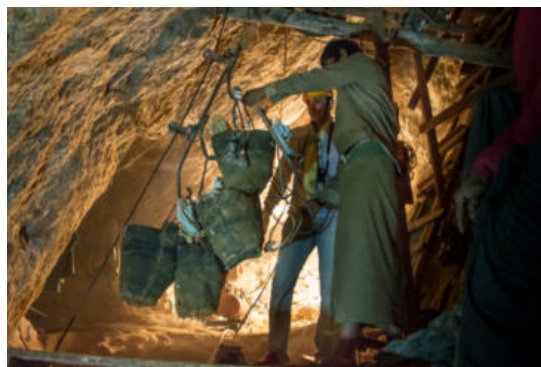
Figure 6. Buckets full of marble are transported to the ore cars using a cable system. Photo by B. M. Laurs.
