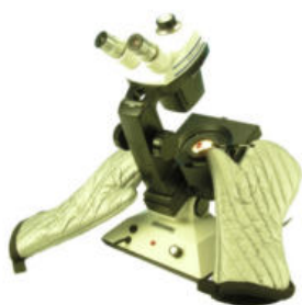
Figure 5. Sustainable LED update of a GemoLite microscope by replacing the darkfield illuminator base and keep the optical system.
