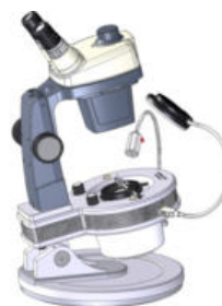
Figure 5. Sustainable LED update of a GemoLite microscope by replacing the darkfield illuminator base and keep the optical system.
