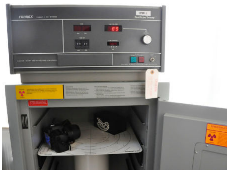
Figure 1. The experiment set up for pearl investigation of X-ray luminescence by using a digital SLR Nikon D90 camera.
