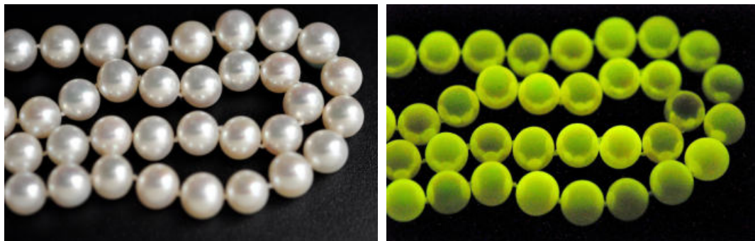
Figure 2. Chinese freshwater cultured red pearl strand recorded under normal light (a), under X-ray radiation displaying distinct green-yellow luminescence (b).
