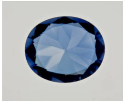
Figure 1. These new synthetic diffused sapphires showed distinct patchy coloration in immersion, making the fairly easy to identify. Mag. 10X, Photomicrograph by Shane McClure.
