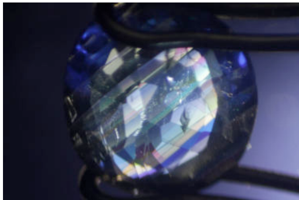
Figure 1. Twin planes in a sapphire from the Kyat Pyin area, Mogok, Burma. - Magnification 5x. Photo: Hpone-Phyo Kan-Nyunt, Gübelin Gem Lab Ltd.
