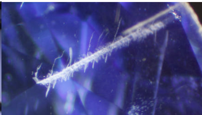
Figure 2. At the intersection of perpendicular twin planes, these intersection «needles», most likely of boehmite (not identified), can be found. - 45x. Photo: Hpone-Phyo Kan-Nyunt, Gübelin Gem Lab
