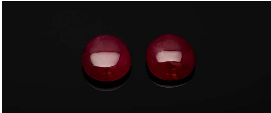
Figure 4: Pair of rubies from Greenland, heated in a borax flux (Photo: Benjamin Huaysan, DSEF).
