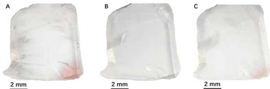
Figure 5. Variation of the red colour zone in the natural red sample (N001-3) before treatment (A), after being quenched from 1170 °C (B), and after being held under 850 °C for 24 hours (C). The red colour faded in (B) and reappeared in (C).
