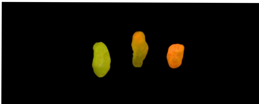
Figure 2: Three cultured freshwater pearls without bead from China under X-rays. The left sample presents yellow-green luminescence, the centre sample presents yellow-green luminescence as well as areas with orange luminescence and the right sample presents principally orange reaction under X-rays. Photos by Hasan Abdulla, DANAT.
