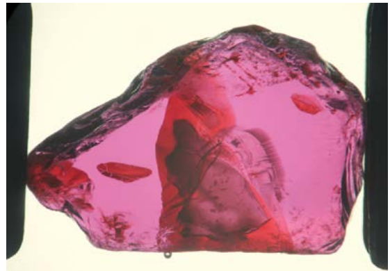
Figure 2: The slice from figure 1 after the low-temperature treatment (900°C, 8h) (transmitted light, image width 11.41 mm). Note the reddish colour of the “natural staining”.
