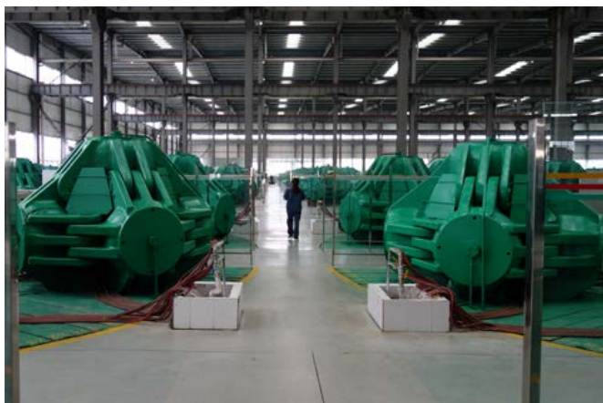
Fig.2 HPHT synthesis equipment of Huanghe Whirl Wind Co. Ltd.. Photo by H. Kitawaki
