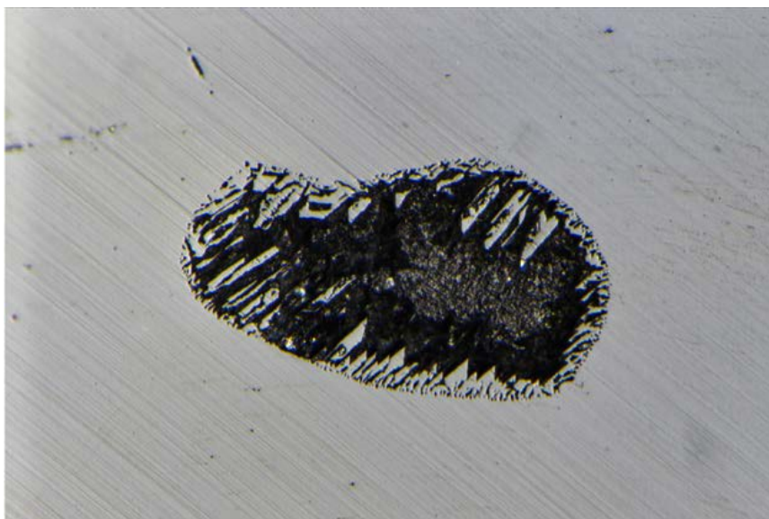
Figure 3. A couple of the samples showed distinct crystallization of corundum around the edges of cavities. F.O.V. 1.59mm. Photomicrograph by Nathan Renfro.
