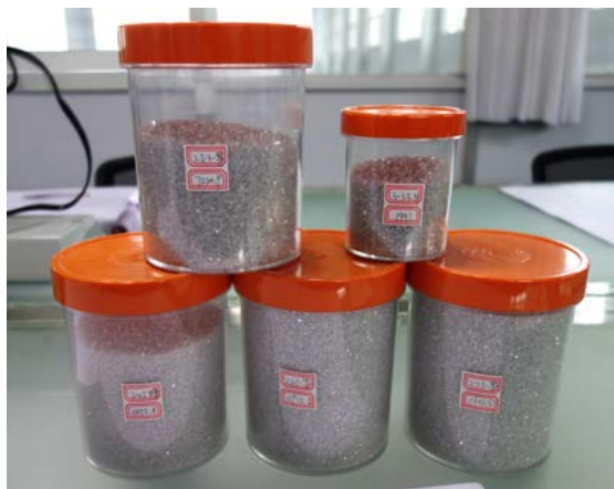
Fig.3 Melée sized rough synthetic diamonds made by Huanghe Whirl Wind Co. Ltd. (five day's production). Photo by H. Kitawaki
