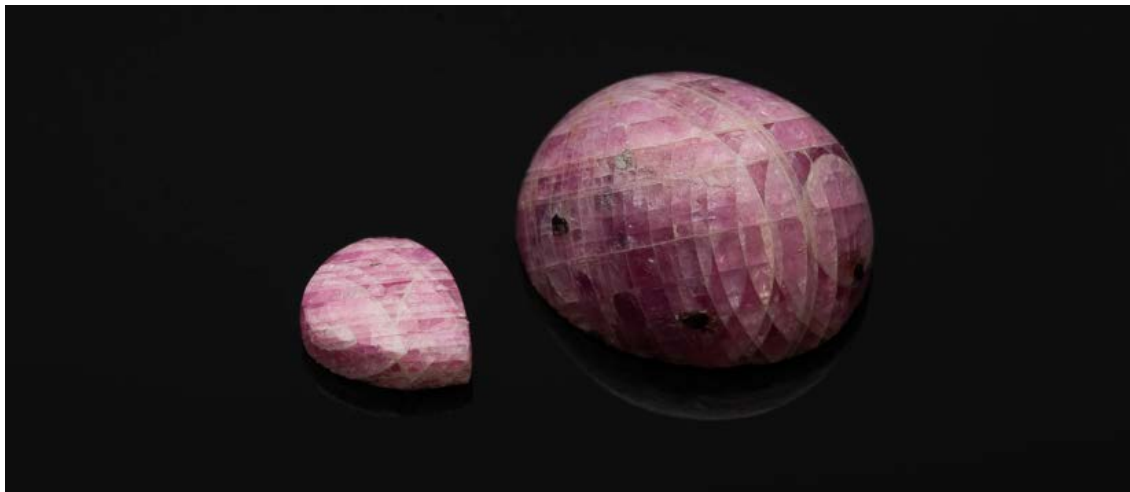
Figure 3: Pink sapphires from Greenland, heated without flux. Note the whitish striation along the twinning lamellae caused by the dehydration of aluminum hydroxides, which form polycrystalline corundum (Photo: Benjamin Huaysan, DSEF).
