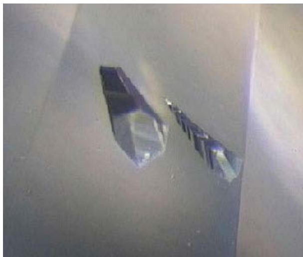
Figure 2: Typical dissolved dislocations in diamond, with a polygonal section, and a tapered shape pointing inside. Photo by Aurélien Delaunay (Field of view about 0.85 mm).
