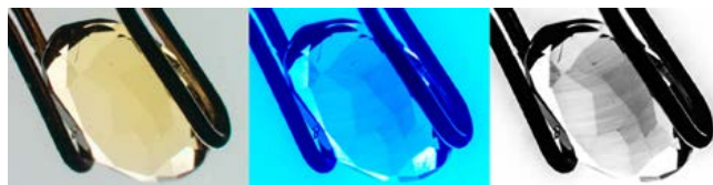
Figure 2. The banding in this yellow Verneuil sapphire becomes visible in blue light and can be accentuated in a post-processed B&W image. Immersed in water. K.E. Fox photo.
