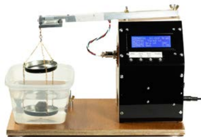
Figure 5. Hundred-gram SG system. K.E.Fox photo.
