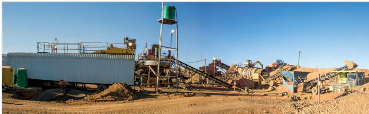
Figure 2. The processing plant at the Tirisano mine employs vibrating screens (centre-right), a scrubber/trommel (right), washing pans (center) and a secure area for X-ray and hand sorting (white container on the left). Photo by B. M. Laurs.
