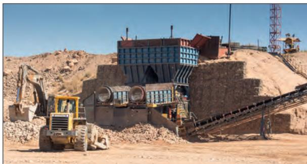
*Figure 5. Trommels are used to remove oversized material at Rockwell Diamonds' Saxendrift mine. Photo by B. M. Laurs.*
