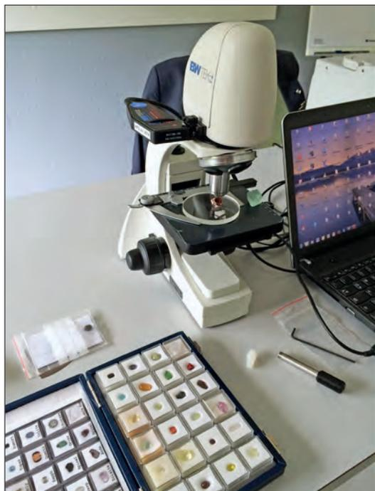
Figure 3. Video Microscope BAC151B connected to the GemRam.
