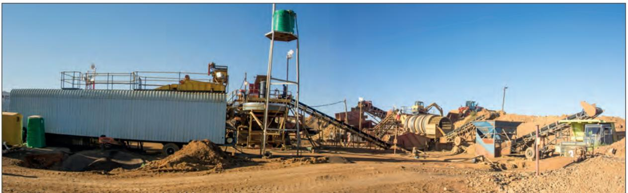
Figure 2. The processing plant at the Tirisano mine employs vibrating screens (centre-right), a scrubber/trommel (right), washing pans (center) and a secure area for X-ray and hand sorting (white container on the left). Photo by B. M. Laurs.
