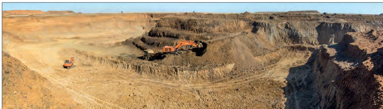
Figure 1. This large open pit at the Tirisano diamond mine is being expanded with excavators and dump trucks. Photo by B. M. Laurs.
