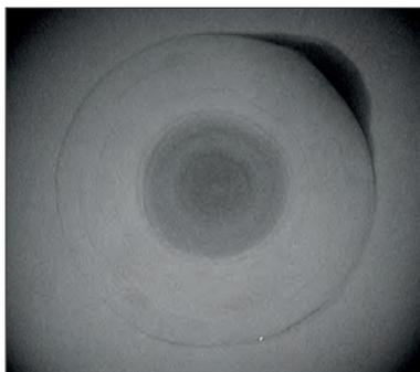
Figure 1b. X-radiograph of the SWCP showing concentric growth lines in the natural *P. maxima* pearl used as bead. A demarcation is observed along with a dark coloured area, due to tissue graft used during cultivation. This demarcation is often seen in CPs with bead.
