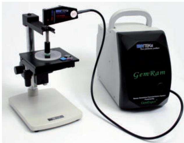
*Fig. 1 The GemExpert Raman probe with sample stage, PC with the identification programme is not shown.*
