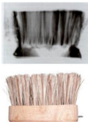
*Figure 1: the “brush effect” in CVD synthetic diamonds: dislocation bunches anchored in the seed plate resemble whisker bunches anchored in the handle of a brush. X-ray topograph courtesy Philip Martineau, DTC Maidenhead, England.*
